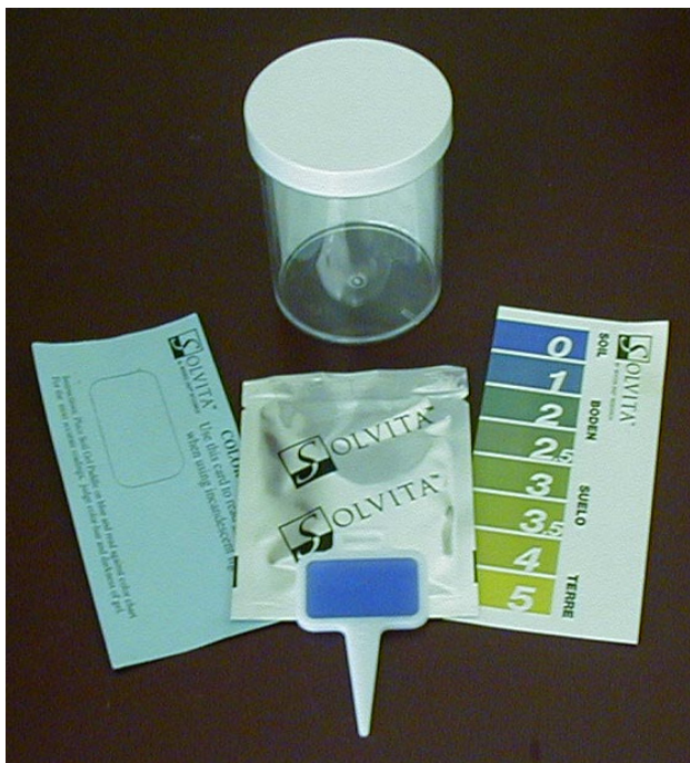
Figure 1. Solvita® test kit: plastic jar, color reading card, Solvita® packet, Solvita® paddle, and color card.
